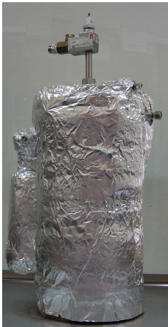
Fig. 2. Appearance of the natural gas fuel processor for the 1 kW class residential PEMFC system, height: 500 mm, diameter: 250 mm.
